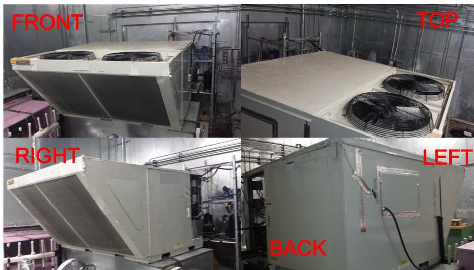
**Figure 4:** Example RTU under testing at OSU psychrometric chambers.
